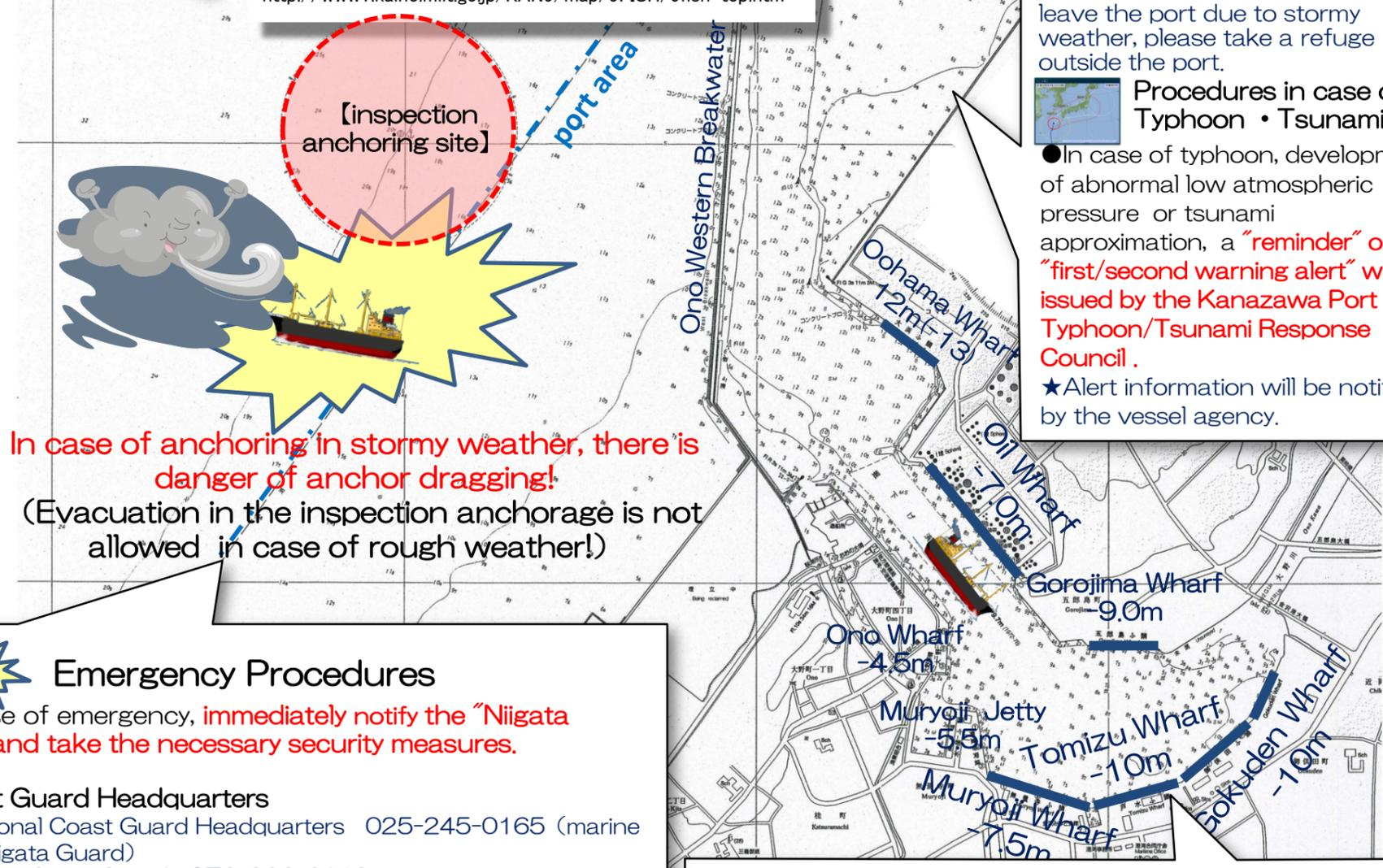
In case of anchoring in stormy weather, there is danger of anchor dragging!
